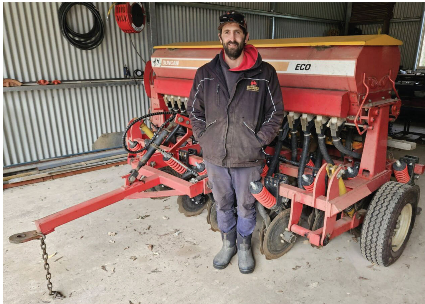
Phil Giancono with his Duncan Drill fitted with RYAN NT retrofit double discs
